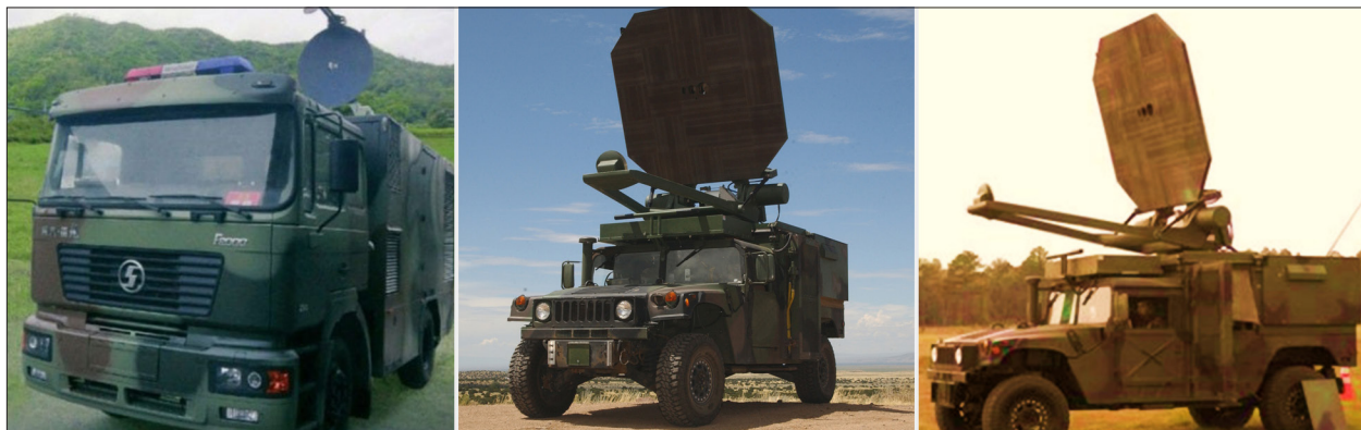
Figure 9: (left to right) A Chinese non-lethal counter personnel system (credit Top81 via IHS Janes); The U.S. Joint Intermediary Forces Directorate Active Denial System, a counter-personnel millimeter wave system; Russian counter-personnel system (Hambling 2012).
